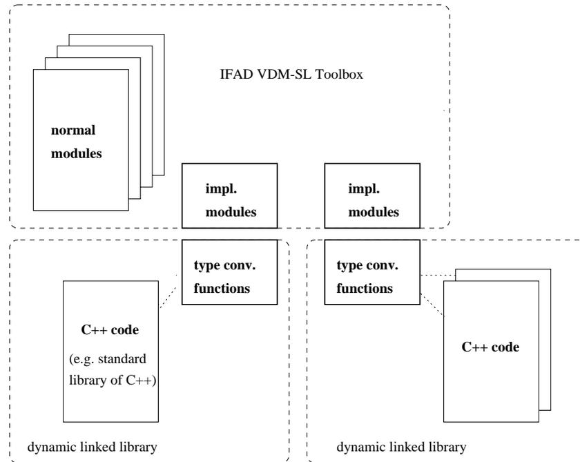
**Fig. 1.** Basic idea of combining code and specification in the Toolbox
